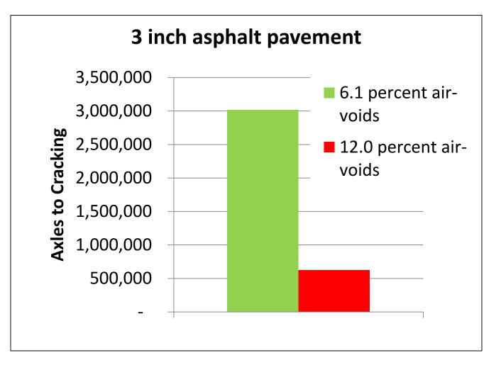
General rule: 1% increase in constructed air-voids = 10% reduction in fatigue life
